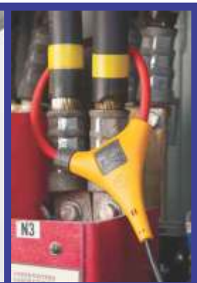
Measure bigger size conductors
